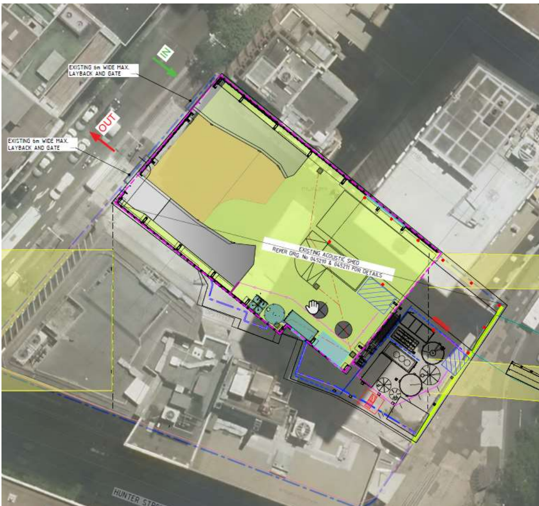
Figure 6: Proposed Hunter Street East Construction Site Access and Egress During Tunnelling Excavation and Lining
